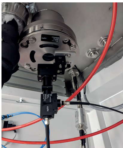
Fig. 1: Photographs of the InspiRe metrology system installed at a PEROvap evaporation chamber at HySPRINT - A Helmholtz Innovation Lab of Helmholtz-Zentrum Berlin. Left: Optical measurement head mounted to the chamber; Right: Glove box containing the chamber with the measurement PC and controller (in black rack compartment) next to it.
