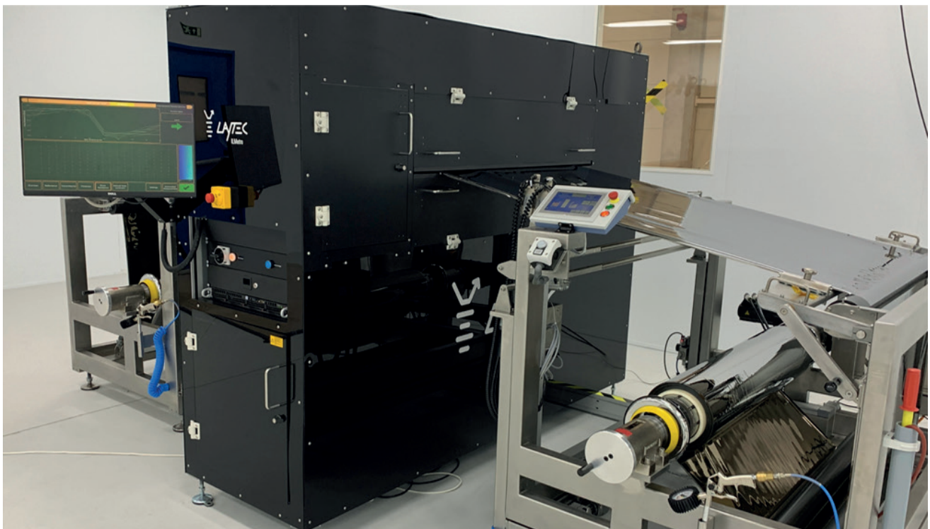
Fig. 1 ILMetro R2R metrology system as recently installed by a leading manufacturer of flexible photovoltaic modules. Here the system is directly integrated into a winder system for transporting the foil to the appropriate measurement positions for quality control purposes.
