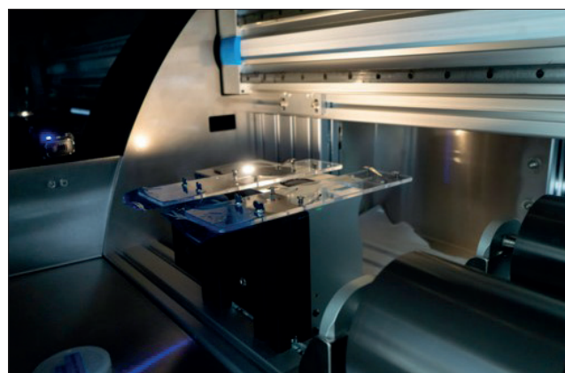
Fig. 2: Separate sample compartment for the manual characterization for small-scale R&D samples.
